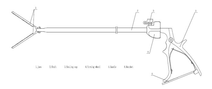
1-2. Jaws of tip 2. Working shaft 3. Sealing cap on irrigating port 4. Turning wheel 5. Handle 6. Ratchet
